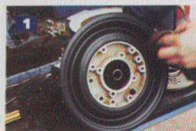
1 New seal in place on gear box. Don't use any sealing compound.
