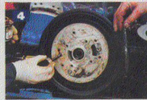
4 Brush sealant on to the clamp plate before fitting the gasket.
