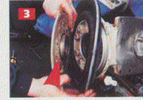
3 Separating the clamp plate and seal from the gearbox. Note the old 'O' ring on the clamp plate.
