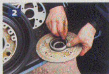
2 New 'O' ring being placed on to the top of the clamp plate.
