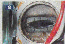
8 The rear of the gearbox and the gearbox plinth waiting for the leg and new seal.
