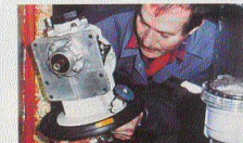
2 Engine has been eased forward (above) leaving a gap between the bell housing and the gearbox, disengaging the drive shaft, allowing removal of the leg and gearbox (right).
