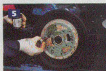
5 Fit the gasket and treat its lower face with the sealant ready for refitting to the gearbox.
