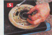
4 Clean clamp ring and remove the old 'O' ring.
