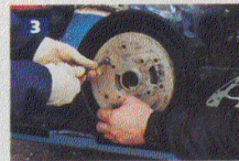
3 Attach the clamp plate with the long and short studs.
