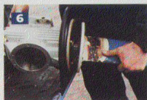
6 The leg being offered up to the gearbox assembly. Don't forget the shim washers!
