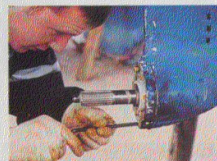
9 Replace the prop shaft and bearing. Fit a new anode and refill with oil.
